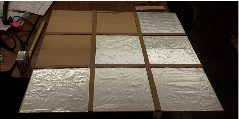
Building the step-on switches made out of wood, cardboard and aluminum foil.
